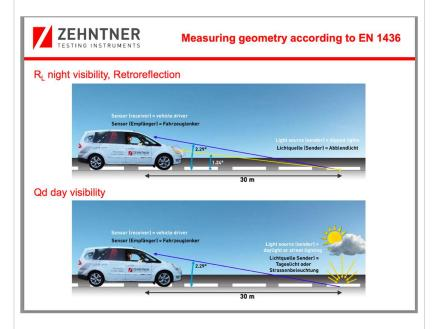
A retro reflectometer is used to measure the retro reflection performance of the surface. The ability of a driver to view the markings, while driving at speed, from a distance, whether in day or night, dry or wet, can ensure avoidance of accidents.
